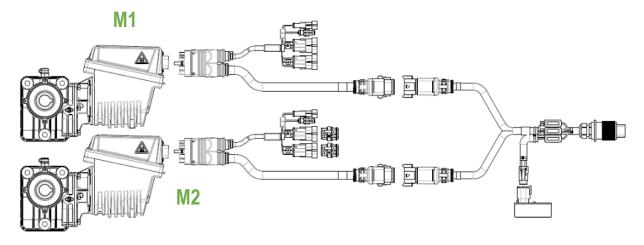
Picture 2-13 Motor wiring diagram on similar applications on the same side (base kit)
