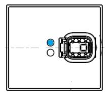
Picture 3-1 Access Point: Blue status LED for Wi-Fi connection
