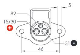
Picture 2-16 ISO 12369 plug on tractor side
