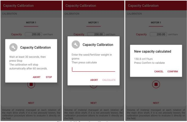
Picture 3-23 Capacity calibration procedure
