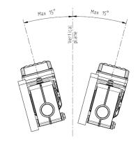
Maximum slope/ angle of the unit As mounted or during continuous operation
