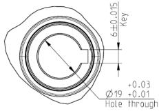
Picture 2-1 Outlet shaft dimensions
