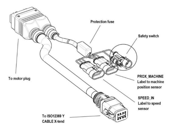
Picture 2-15 X-tend DMD Cable wiring diagram
