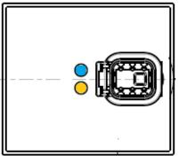
Picture 3-2 Access Point: Orange CAN bus connection status LED
