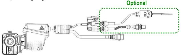
Picture 2-5 Speed sensor connection option
