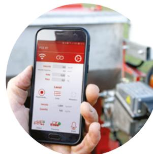
The seed quantities required and product density were entered as indicated by the app for controlling the Agri-Motion PCS W1 system. After calibration of the sensor for speed and the cubic centimetres of the distributors per revolution, the work was completed without any problems because the quantities deposited on the ground had been pre-set.
