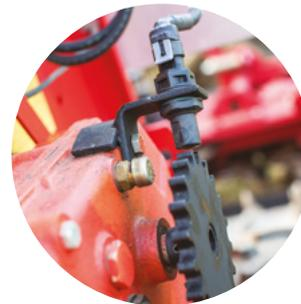
To read the machine travel speed, the magnetic sensor supplied was used and a 4-mm thick phonic wheel was created.
