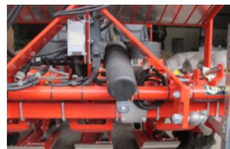
A **magnetic encoder** fixed to one of the transplanter wheels, provides an accurate speed reference to the motor, ensuring the precision even at low speeds.
