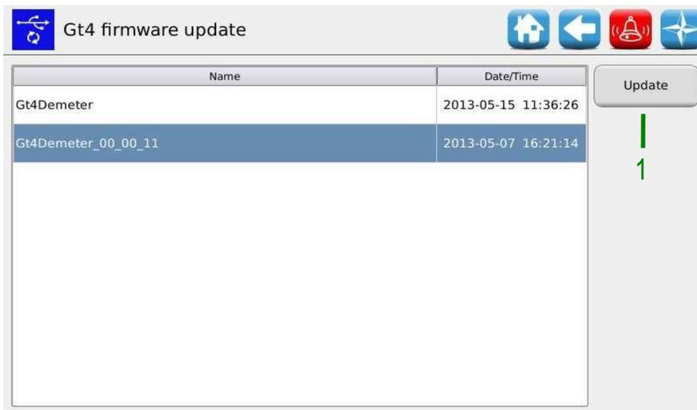
Selecting the desired SW from the list and pressing the **1** button it is possible to update the HMI.
